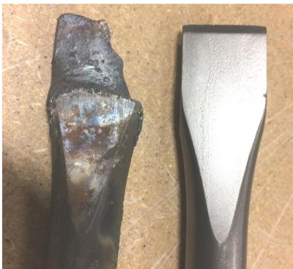
**\*\*INCIDENT 10/8/18** This was in a parking garage. If you see a "cover plate" (picture on left) you need to stop what you are doing and find out what it is covering. Picture on right shows the chisel after it came in contact with the live electrical wiring inside a conduit compared to a new chisel.
